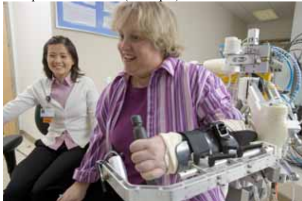
Fig. 1. Person with a stroke participating in movement training with a robotic exoskeleton called Pneu-WREX. This pneumatic robot allows motion of the arm in four degrees-of-freedom (DOF). The robot allows the hand to reach a wide range of points in 3D space, but with the forearm always horizontal. The device allows a small amount of shoulder translation forward and backward.
