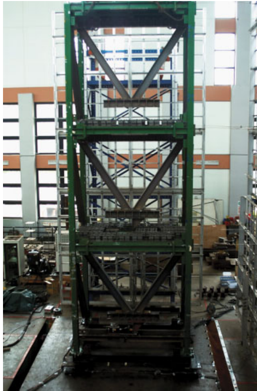
Figure 10. Three-storey large-scale frame model on shake table.
