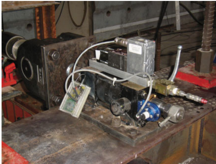
Figure 5. RSASD connected to an actuator.
