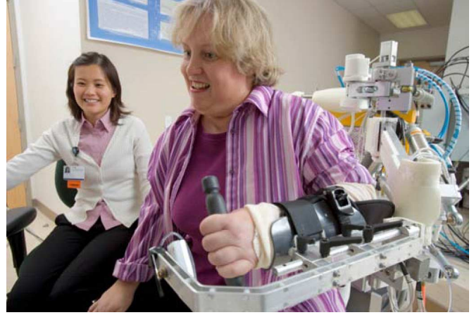
Fig. 1. Pneu-WREX: A four degree-of-freedom pneumatically actuated upper extremity orthosis for robot-aided movement training.
